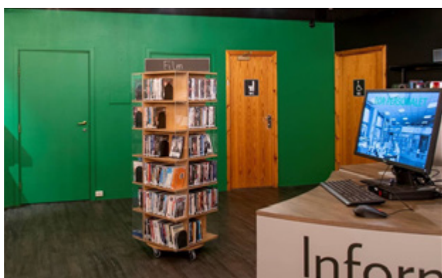
After: doors concealed with same colour as the wall, new toilet sign and the information desk has been marked.
